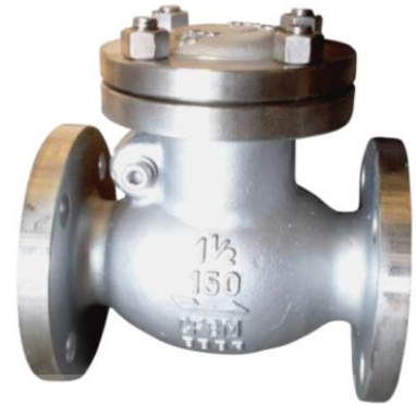
ANSI 150# SS316 Flange End Swing Check Valves
